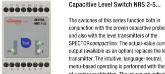
conjunction with the proven capacitive probes and also with the level transmitters of the SPECTOR*compact* line. The actual-value current output (available as an option) replaces the level transmitter. The intuitive, language-neutral, menu-based operating is performed with the aid of a rotary pushbutton. The values are indicated on a 4-digit 7-segment display. The 100% range setting can be made from a filling level of 25%.
